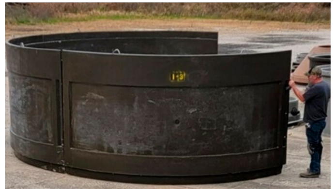
Figure 2. Precast polymer concrete tunnel reline segments. Washington, Indiana Plant
