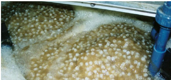
We designed, constructed, and are operating an aerobic biological treatment system for the biodegradation of 1,4-dioxane at the Lowry Landfill Superfund Site in Aurora, Colorado.
