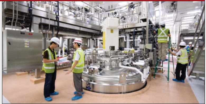
LBXS1 fermentation suite containing 20,000-liter bioreactor with operators commissioning the system
